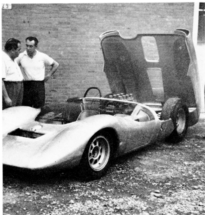
Fantuzzi and de Tomaso discuss the just-completed prototype. Rear cover provides access to wheels as well as engine.
