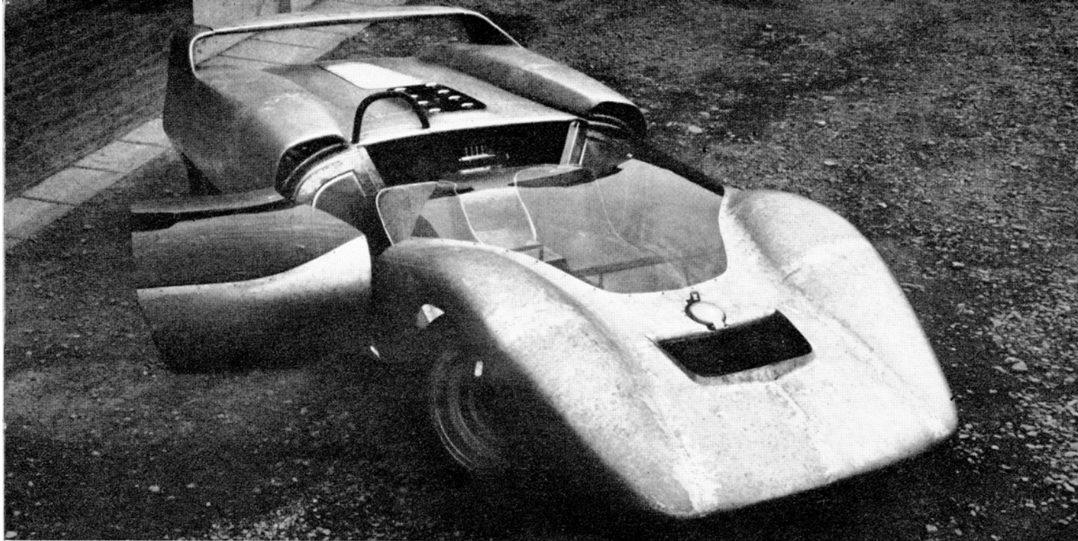
Completed, but not painted, prototype showing regulation GT doors, air intakes away from skin for airflow considerations.
